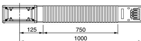
**EDF - Flexible length, 3 m for detours around obstacles - IP55**
