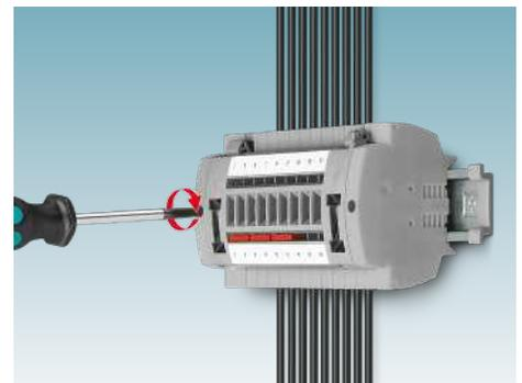
The preassembled test terminal strips can be mounted in a space-saving way in the control cabinet by simply snapping the E-UTWE 6 adapter onto standard NS 35 DIN rails.
