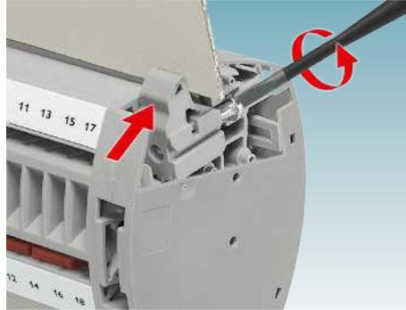
The patented panel fastening is easy to use and has a robust design. Large tolerances in the sheet metal cutout of up to 4 mm are compensated for by the eccentric tappet function.
