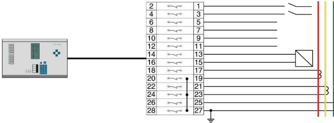
**Plug-in test socket for 19" rack or wall mounting, with current transformer, voltage transformer, and signals**
