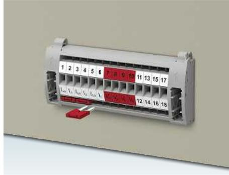
Automatic, leading transformer short circuit implemented with standard plug-in bridges in the plug-in test socket. The positioning of the short-circuit bridges on the outside of the control cabinet is clearly visible.
