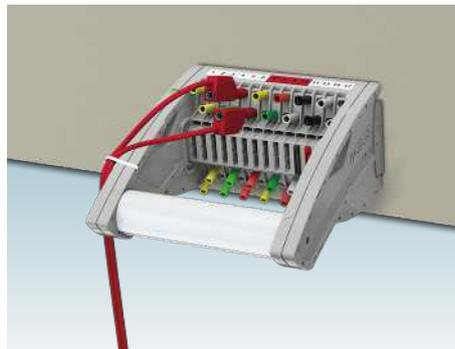
Space saving with offset test socket arrangement. The test cables can be easily fixed in place with cable ties.
