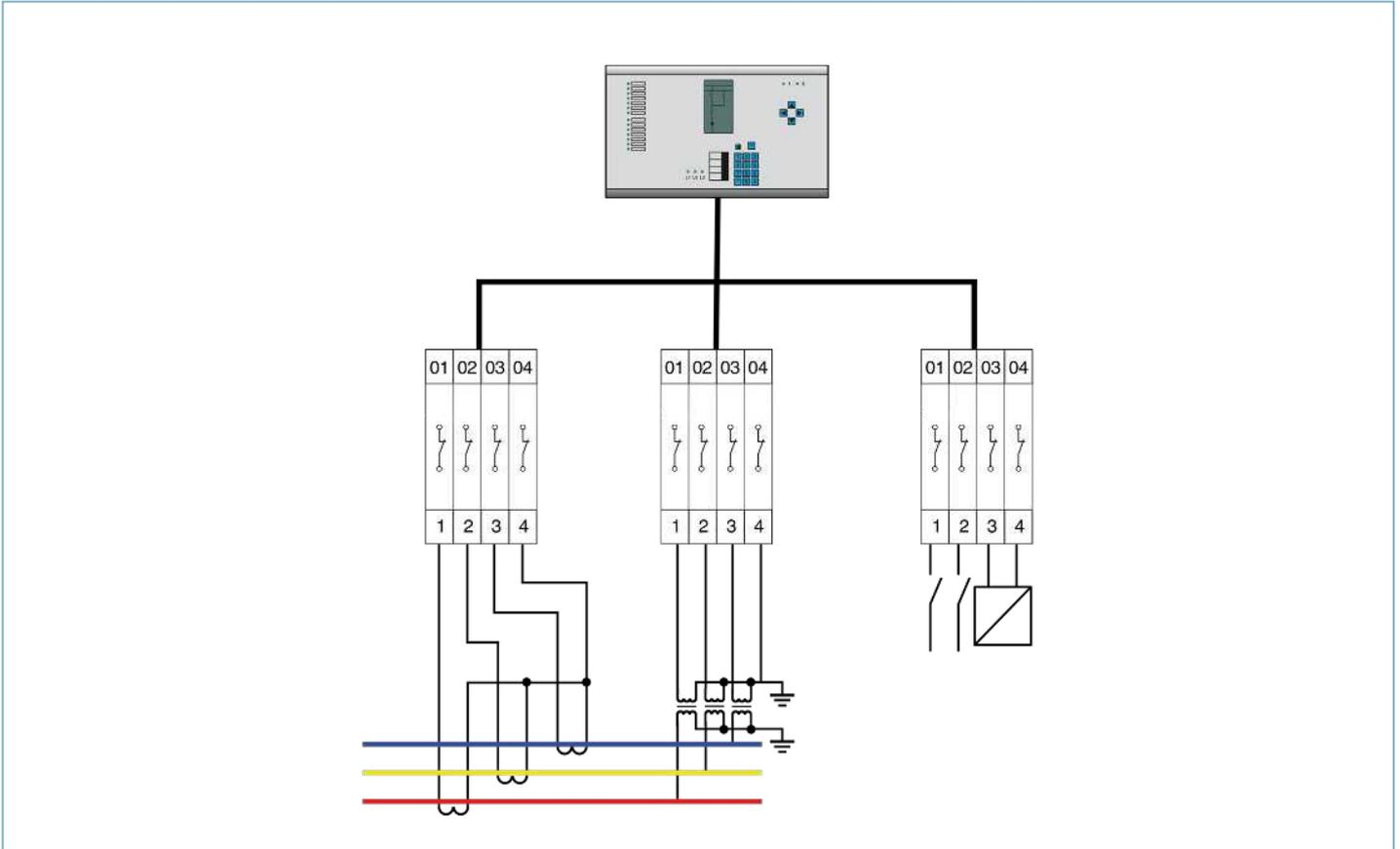
**Plug-in test socket for current transformers**
