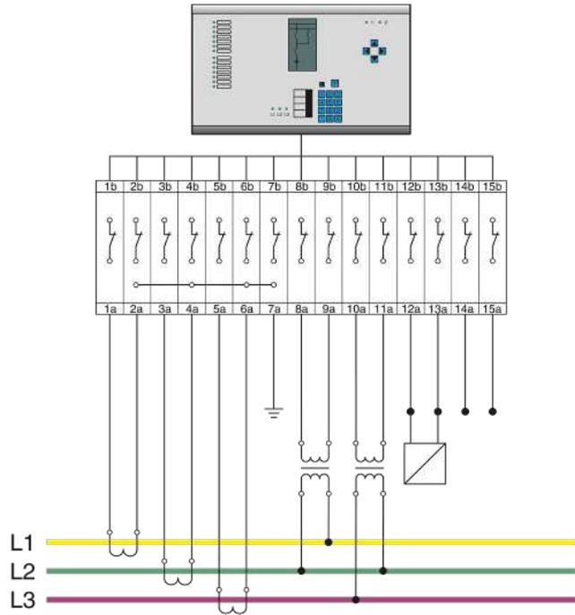
**Plug-in test socket for DIN rail mounting with current transformer, voltage transformer, and signals**
