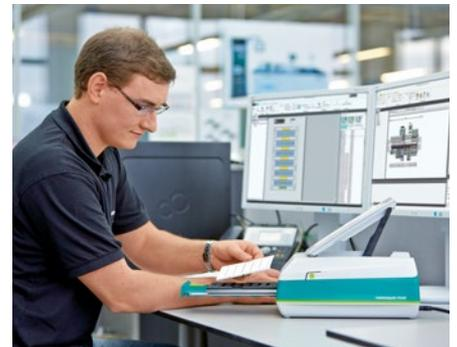
In stationary use, the THERMOMARK PRIME can be easily controlled and managed via the MARKING system software. The mobile printer has integrated software for identification on site.
