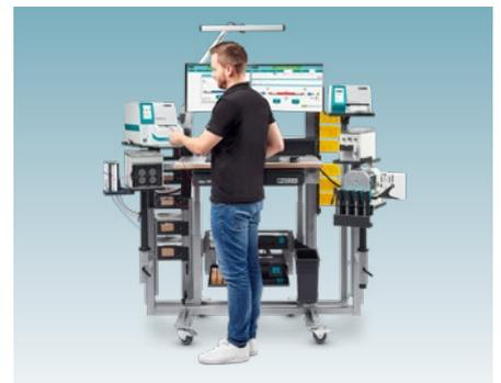
The clipx WIRE assist worker assistance system enables efficient wire processing. Combine the software-supported system with your printing systems for easy and ergonomic wire preparation.
