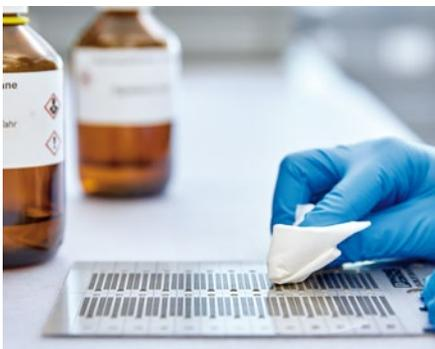
Aggressive cleaning agents can corrode the markings and cause the material to fade, the text to become illegible, or result in brittle fractures. Marking materials must therefore have a high resistance to chemicals.
