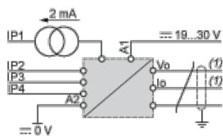
The input, output and power supply lines must be kept away from the power cables to avoid effects due to induced interference.
