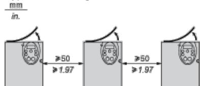
By removing the protective blanking cover from the top of the drive, the degree of protection for the drive becomes IP21. The protective blanking cover may vary according to the drive model, see opposite.
