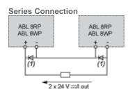
(1) Two Shottky diodes Imin = power supply In and Vmin = 50 V Parallel Connection
