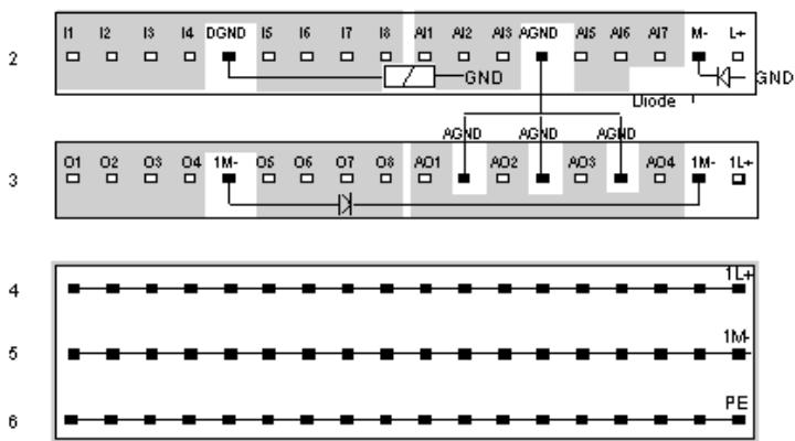
NOTE: AGND and DGND are separated inside the module. External digital inputs must be returned to the DGND terminal. External analog circuits must be returned to AGND terminals.
